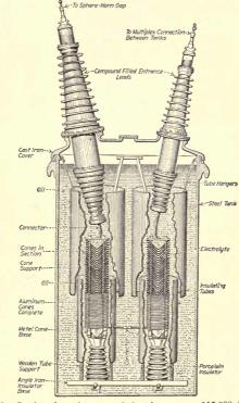
Fig. 176.—Section through a general-electric-company 115,000-135,000-volt electrolytic arrester tank.
